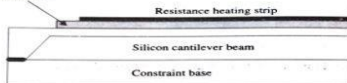
Figure 2.17 | Microactuation using shape memory alloys.
